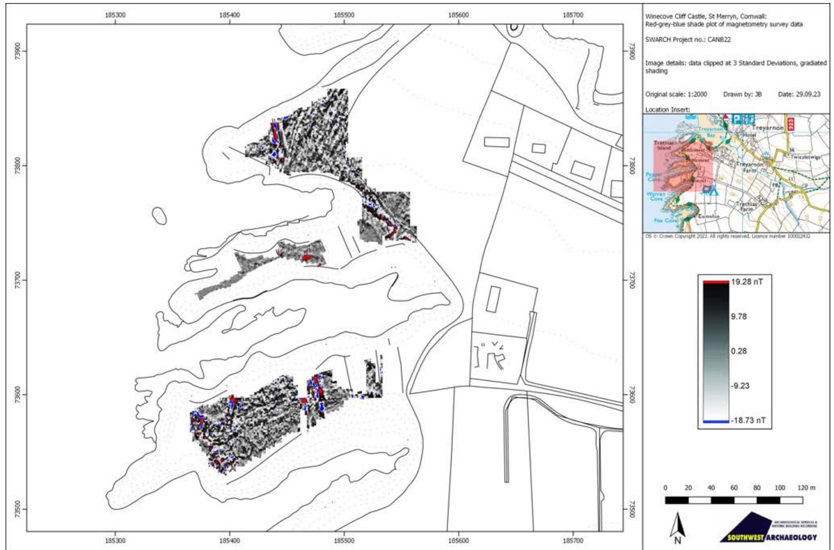
FIGURE 9: RED-GREY-BLUE SHADE PLOT OF MAGNETOMETRY SURVEY DATA; CLIPPED AT 3 STANDARD DEVIATIONS (SD).
