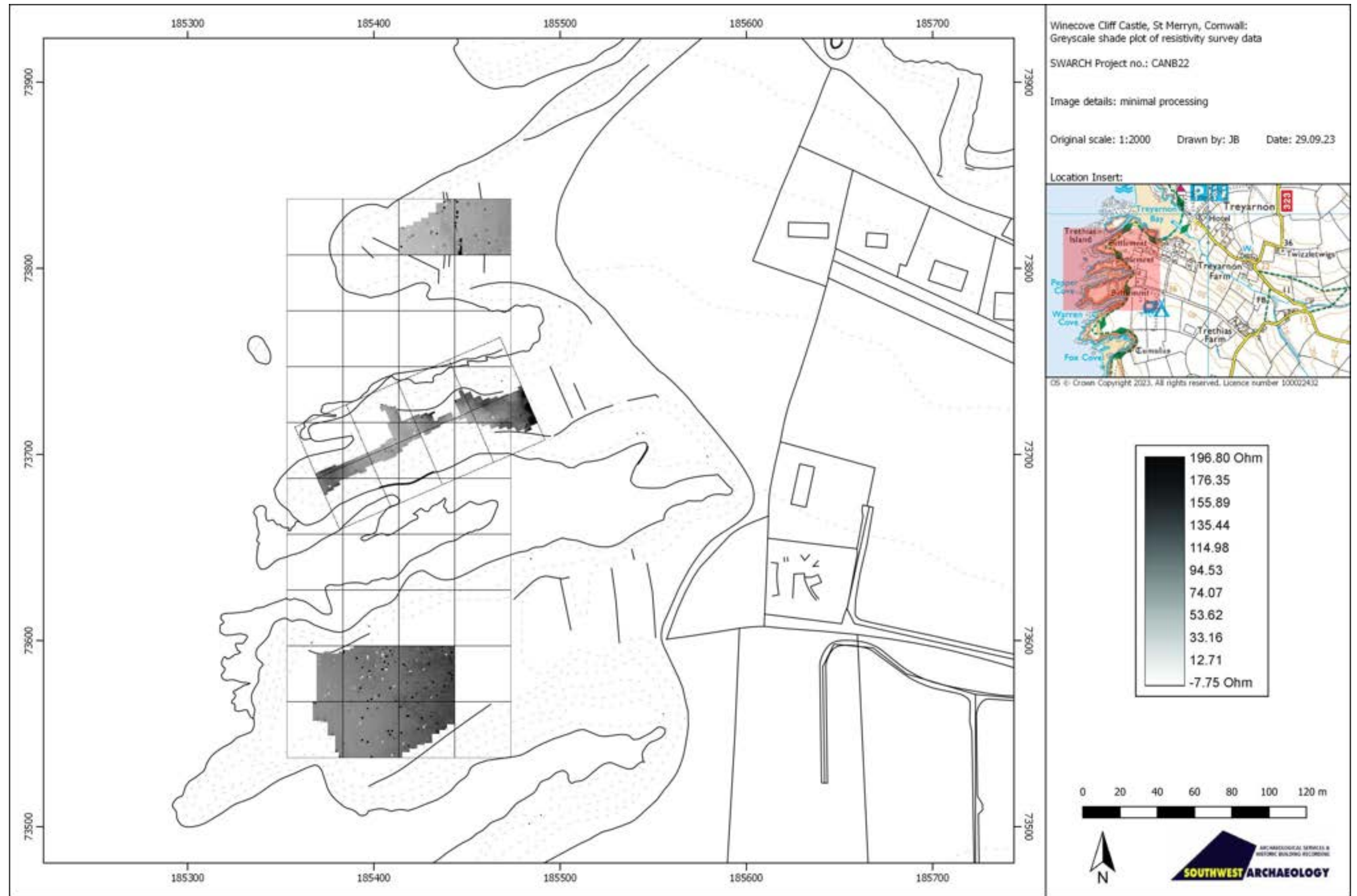
FIGURE 5: GREYSCALE SHADE PLOT OF RESISTIVITY SURVEY DATA; MINIMAL PROCESSING.
